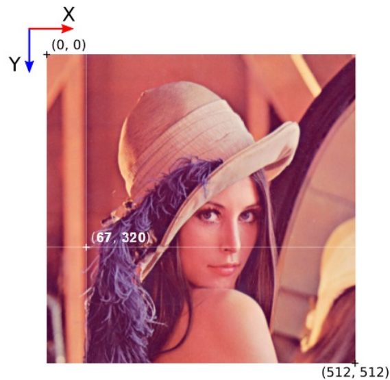
Directions and pixel positions in image coordinates.
