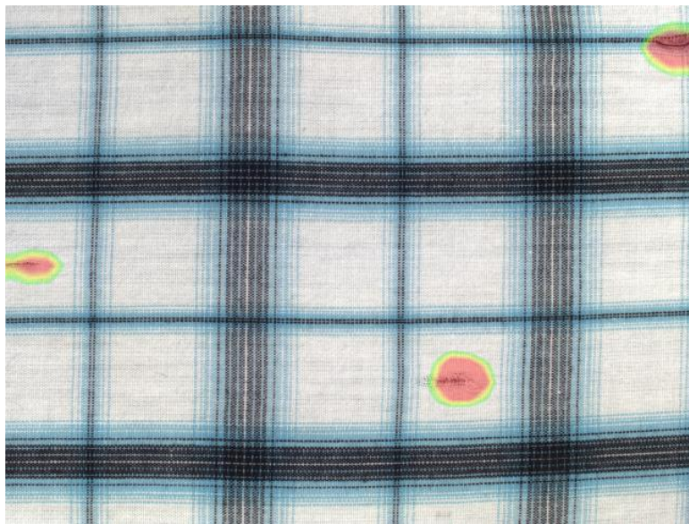
An example of textile defect detection using the AvsFilter_DL_DetectAnomalies2 .
