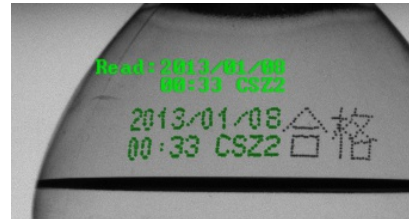
Result of data extraction using OCR.
